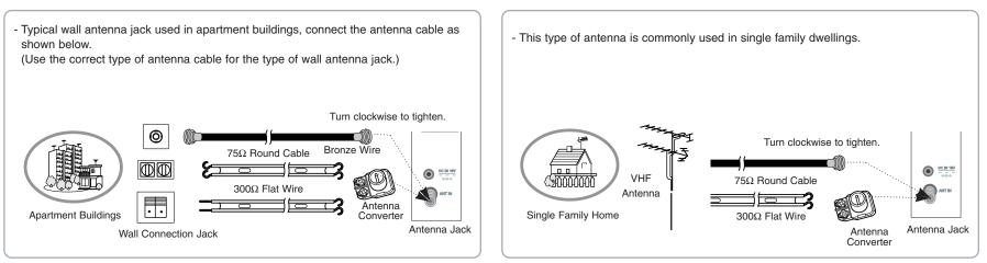
Connecting to an Outdoor Antenna Setup
